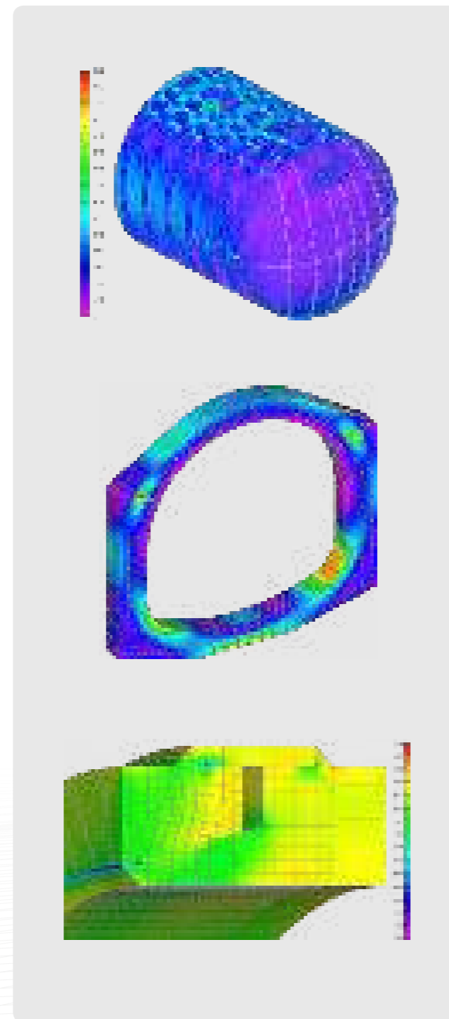
Views of containers, jaw-shaped profiles and welds in the FE model
